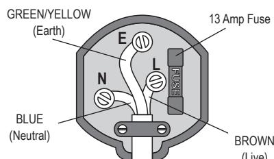
Ensure that the outer sheath of the cable is firmly held by the clamp
